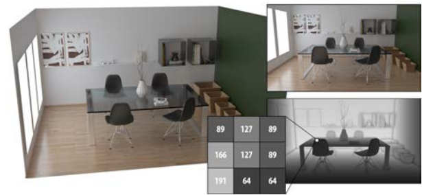
Fig. 1. Color and depth buffer of a 3-D scene, both represented with values in [0, 255].
