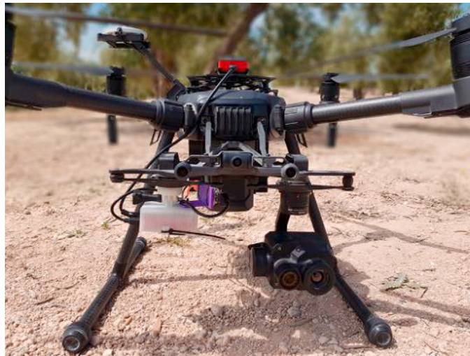
Figure 1. Unmanned aerial vehicle (DJI Matrice 210 RTK) and a thermal camera (DJI Zenmuse XT2).
