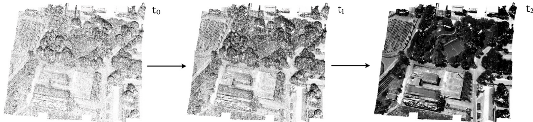
Fig. 8. Iterative rendering of a hyperspectral point cloud during several frames, using 10k points per frame.
